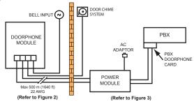
Figure 1 - System Connection
