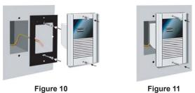
**Note**: To ensure the correct fitting of the Doorphone, please do not allow the screw head to protrude more than 3mm (1/8") beyond the interface bracket.
