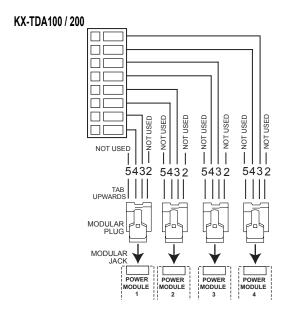
Figure 7 - KX-TDA100/200: Connection Details
