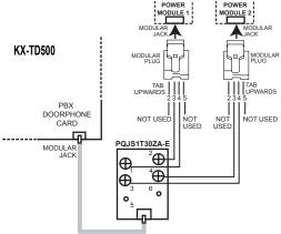
Figure 5 - KX-TD500: Connection Details
