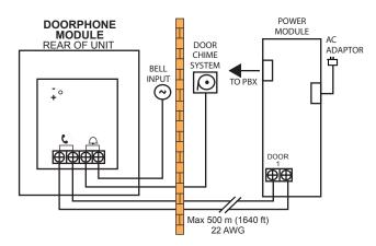
Figure 2 - Doorphone Module's Interconnects
