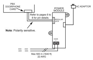
Figure 3 - Power Module's Interconnects
