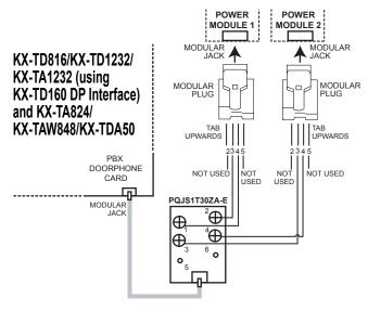
Figure 6 - KX-TD816/KX-TD1232/KX-TA1232 (using KX-TD160 DP interface) and KX-TA824/KX-TAW848/KX-TDA50:
